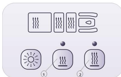
Picture 12 - View of the heating and LED control panel
