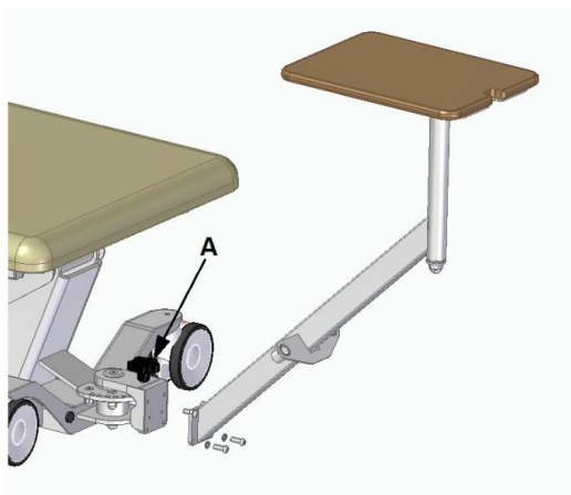
Picture 8 - Attaching and replacing the traction unit base arm of the TRITON 6M traction table.
